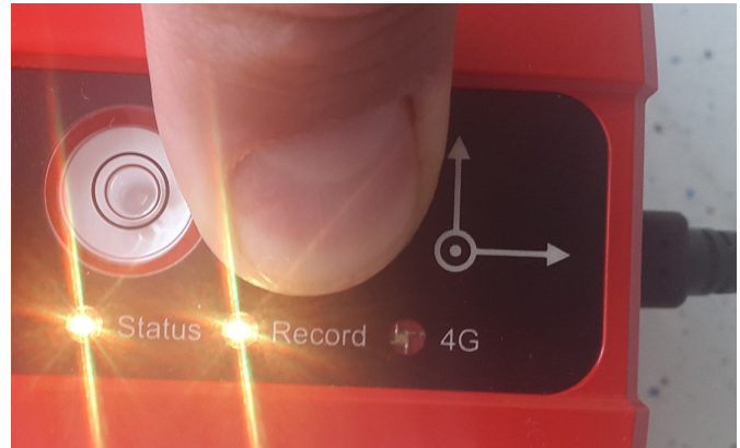
Figure 2. Button pushed for around 10 seconds until the LEDs Status and Record are ON.
